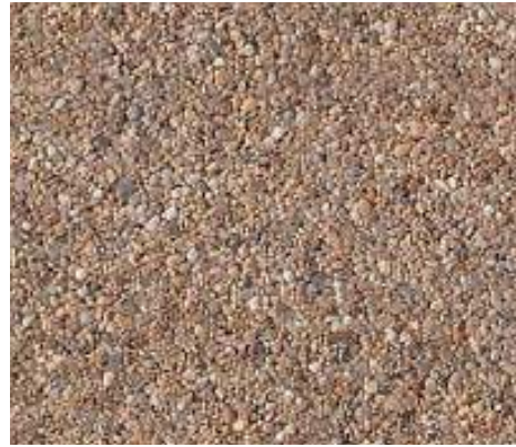
Proposed deck surfaced in natural aggregate resin bound material
