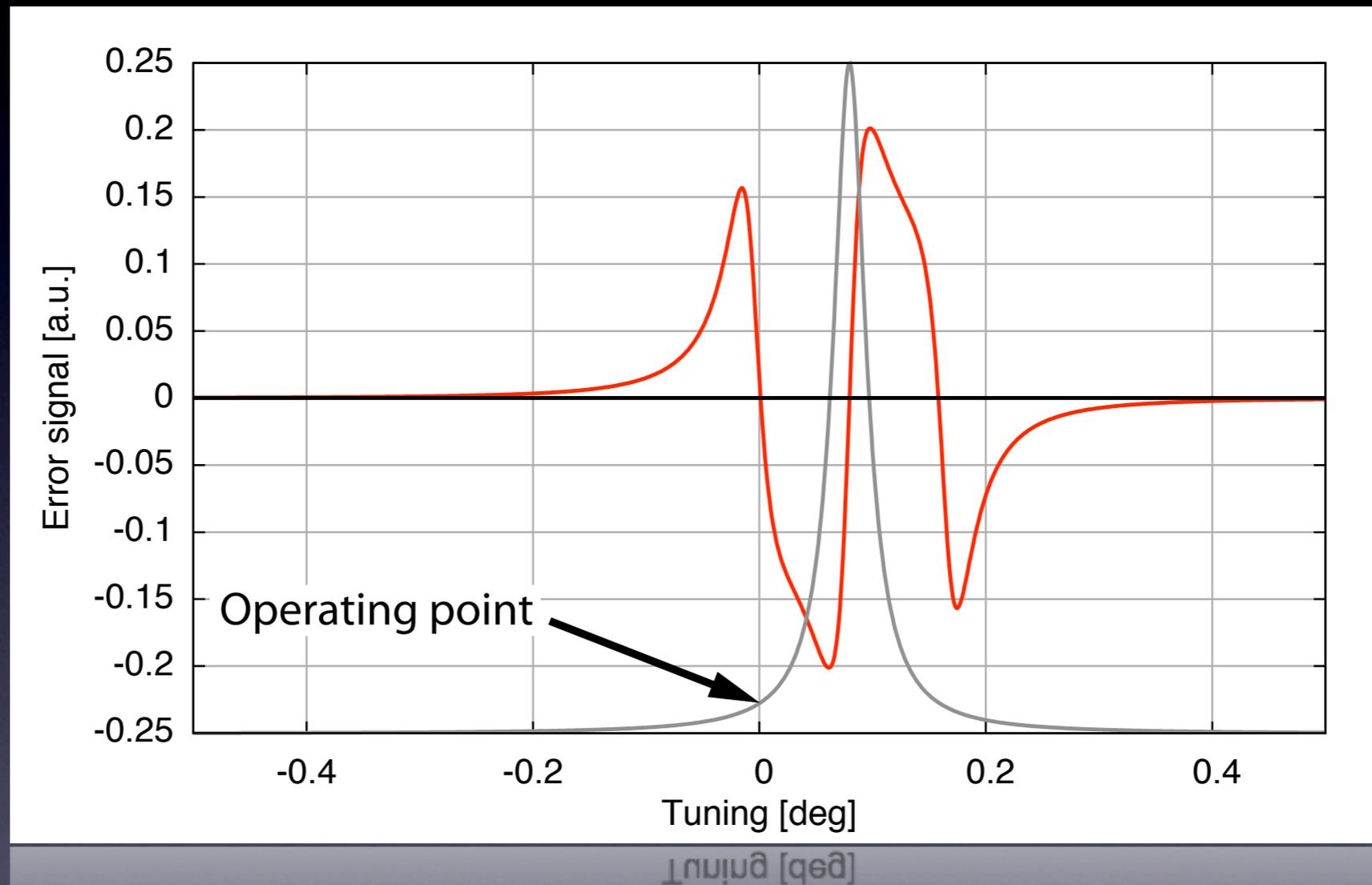
The error signal requires an adaptation of the modulation frequency ( $f_{\text{mod}} > f_{\text{res}}$ ) and demodulation phase
