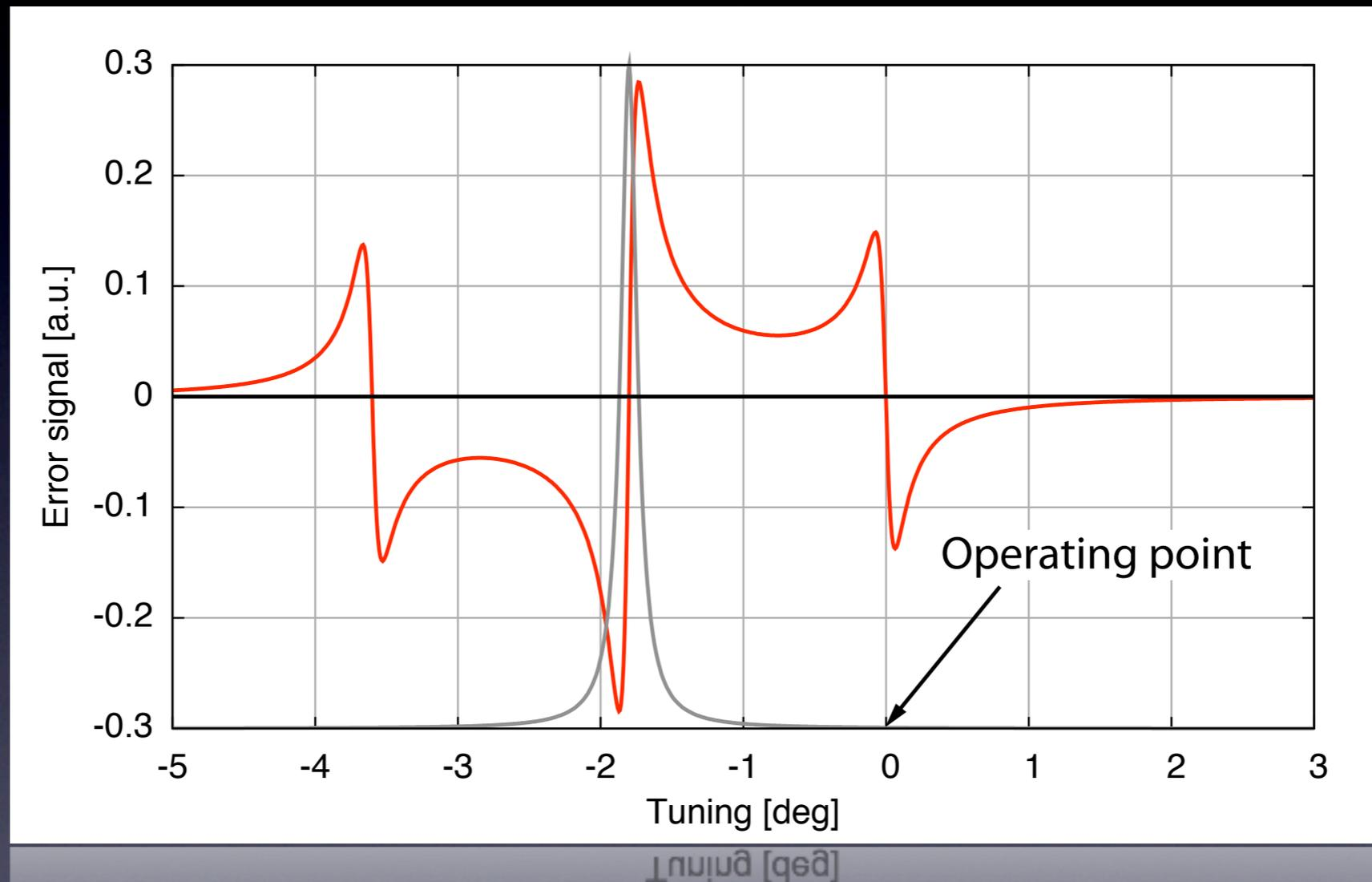
Lock on the zero-crossing corresponding to the resonance of one sideband. This works if  $f_{\text{res}}$  is much bigger than the cavity's half-bandwidth
