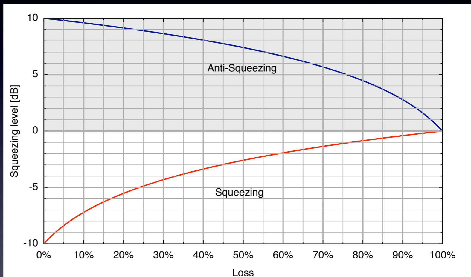
A cavity reflectance  $R < 1$  means loss. The degrading of squeezing is then frequency dependent
