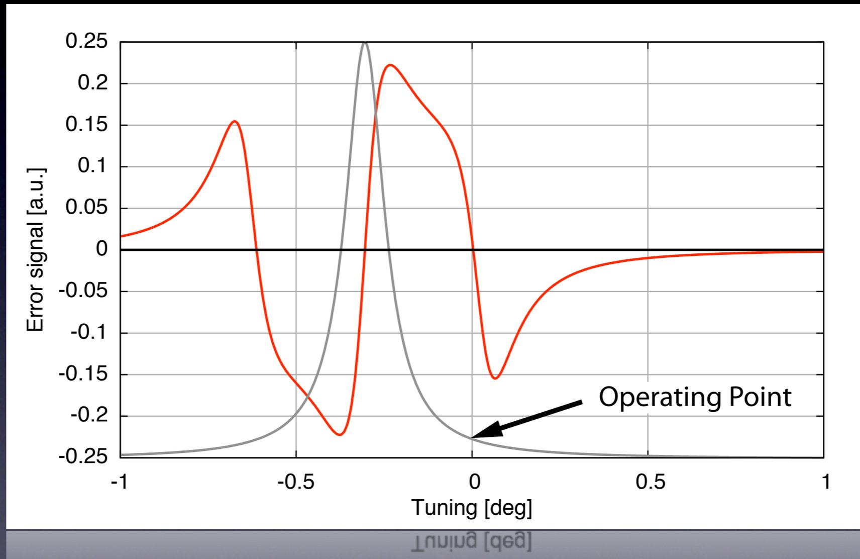
The error signal requires an adaption of the modulation frequency ( $f_{\text{mod}} > f_{\text{res}}$ ) and demodulation phase
