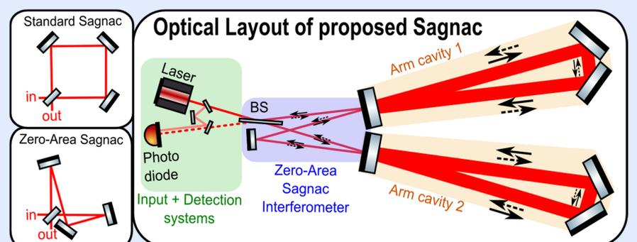
Figure 3: Optical layout of the Sagnac interferometer, which consists of three main building blocks: The input and detection optics including homodyne detection (green), a central Sagnac interferometer (blue) and two high-finesse arm cavities (orange).
