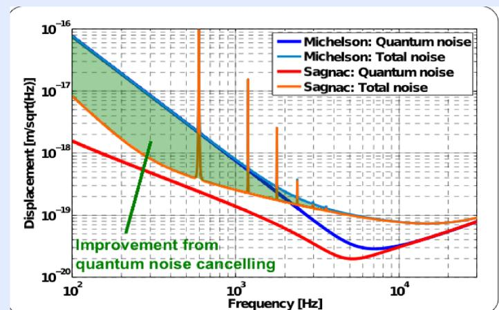
Figure 2: Noise budgets of a Michelson and a comparable Sagnac interferometer (left), both featuring 1gram test masses, arm cavities and a circulating optical power of 1kW. The plot illustrates the improvement in overall sensitivity (green area) that can be achieved by the Sagnac speed-meter over a Michelson interferometer with comparable parameters.
