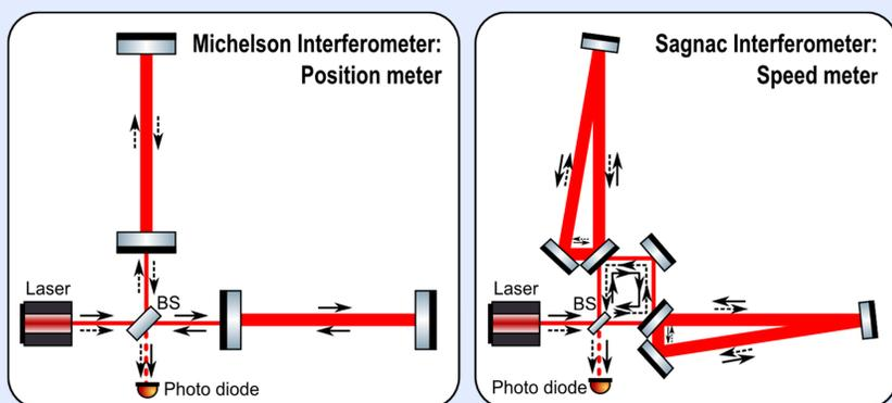
Figure 1: Simplified layouts of a Michelson interferometer with arm cavities (left), which measures the position of the mirrors and a Sagnac speed-meter (right), which measures the momentum of the test masses. In the Sagnac interferometer all mirrors are sensed one time by the light being transmitted through the BS and then a second time (either shortly before or after) by the light reflected from the BS.
