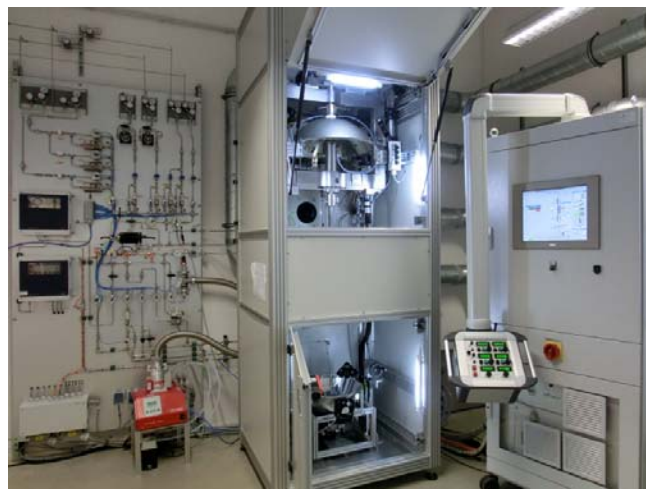
HKZ Scidre Mirror furnace – up to 150 bar O_2 - dedicated for high oxidation state materials -
