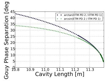
The photodiodes need to be aligned to within around  $4^{\circ}$  at the longest cavity length.
