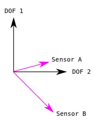
The sensors and the actuators can be represented as vectors in the DOF space.
